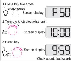
Note:1. The power level is displayed in the percent. With each pressing of the key MICRO the power level reduces from p100 to P80 to P70to P60to P50 to P40to P30 to P20 then start again from P100.
